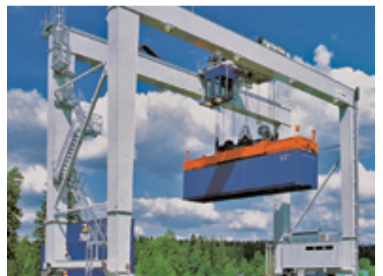
Rubber tyred gantry crane.
